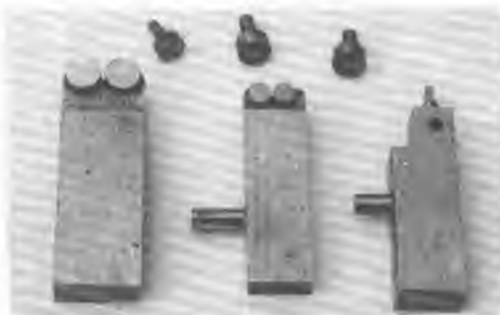
Fig. 91 This shows two button cutters and a "topping tool". The cutters with the pins in their shanks are for use with the 'Eureka' form relieving device. The buttons in the top of the photograph have been hardened and are ready for grinding.
